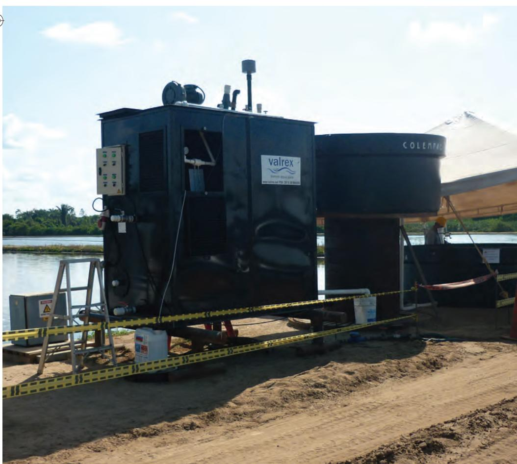
were used to design the full-scale system, which was capable of treating up to 11,400 m<sup>3</sup>/d of gasoline-contaminated groundwater. The full-scale system achieved compliance levels within one week of startup.
