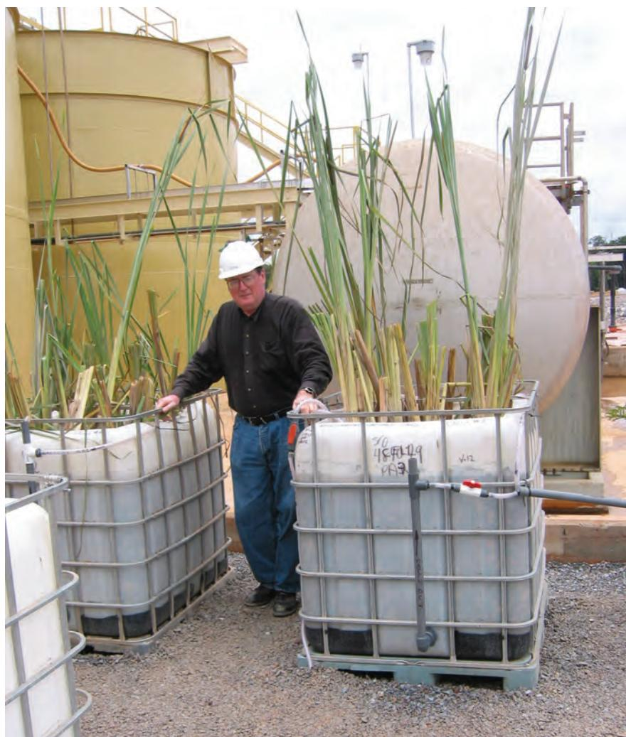
A goldmine in South America needed a low maintenance system to treat ammonia. The test above helped determine the proposed systems abilities and properly size the final product for their needs.
