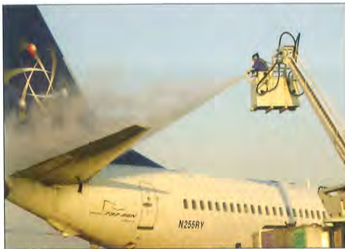
Airplane deicing practices have made air travel safer during cold, winter months. Photo by Rick Reeter, Dallas Ft. Worth Airport
