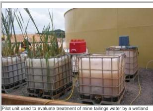
Pilot unit used to evaluate treatment of mine tailings water by a wetland system.
